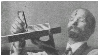
Fig. 105. Testing from Edge to Edge.
