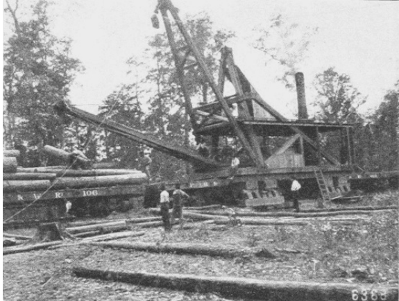
Fig. 27. Steam Skidder at Work. Grant County, Arkansas.
