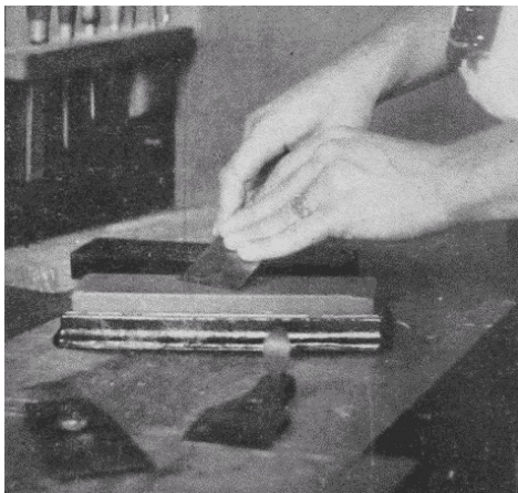
Fig. 77 Whetting a Plane-Bit.
