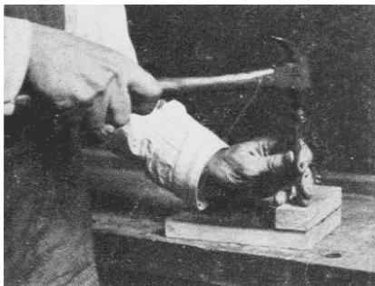
Fig. 165. Using a Nailset.
