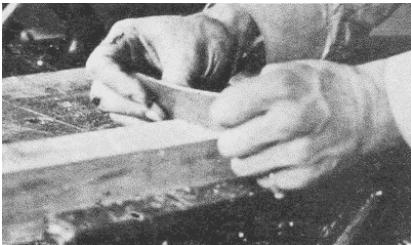
Fig. 152. Using a Cabinet-Scraper.
