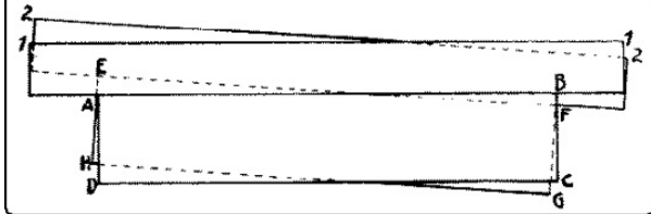
Fig. 206. Method of Using the Winding-Sticks.
