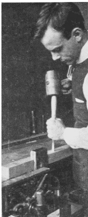
Fig. 76. Mallet Chiseling. The Piece is Clamped Down on the Bench With the Bench Hook.
